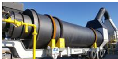
Figure 4 - Vulcan Systems - Dryer & Bag House
